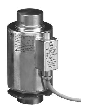
Load cells with type of protection flameproof enclosure "d" are characterized by the fact that they can be used in the corresponding zones 1 and 2 directly and without any additional devices (such as required for power limitation in EEx i).
