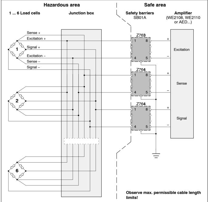
In accordance to the values of inductivity and capacity specified in the certificate of conformity, the following cable length limits between the safety barriers and the junction box are permissible with HBM cable type KAB8/00-2/2/2 (blue):
